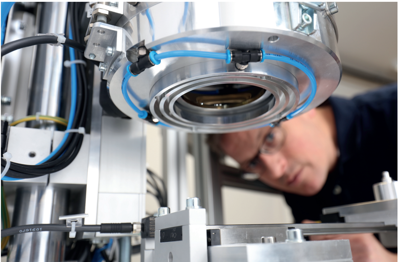
View inside an Evosys laser welding system © Evosys
